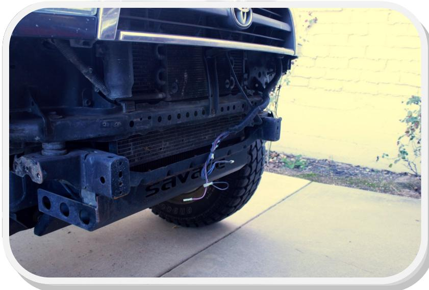
3. If desired, mask off the body and paint your frame rails and the area behind the bumper to hide the "ugly."
